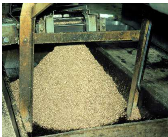
Free-machining brass swarf being collected at a typical machine shop
