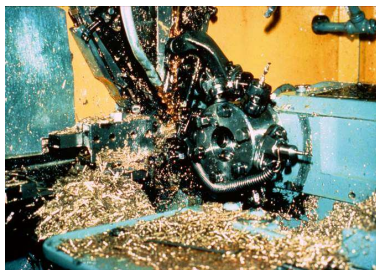
Small fragmented machining swarf literally flies away from the cutting tool during high-speed machining of free-machining brass
