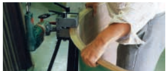
Machine forming of curved trays.
