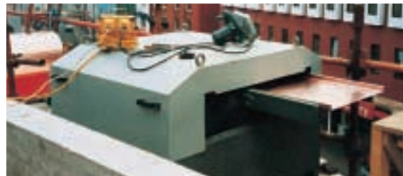
Mechanised Long Strip tray formation from rolled copper sheet.
