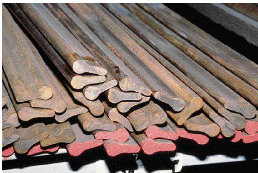
Plate 22 - Rotor Bars made of Copper-Chromium-Magnesium (Vin Callcut)
