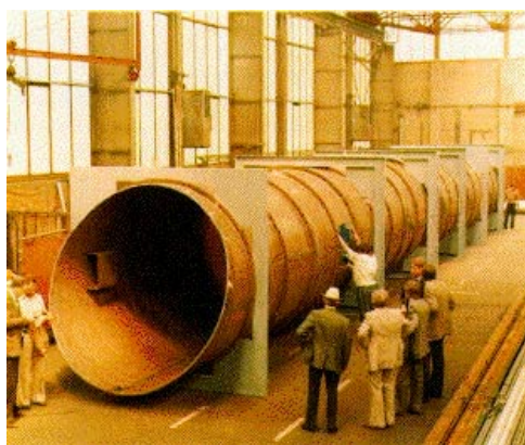
Figure 5 - Seawater suction pipe for the fire extinguishing plant at Jeddah airport in Saudi Arabia.(photo: VDM).
