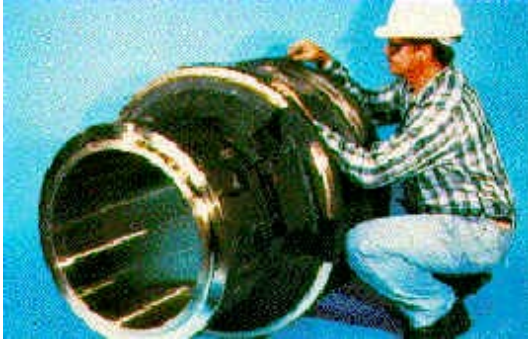
Figure 9 – This marine tailshaft bearing is over 0.5 metre in diameter
