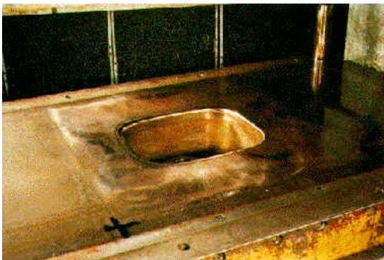
Figure 12 – Aluminium bronze tooling was used to form components such as this
