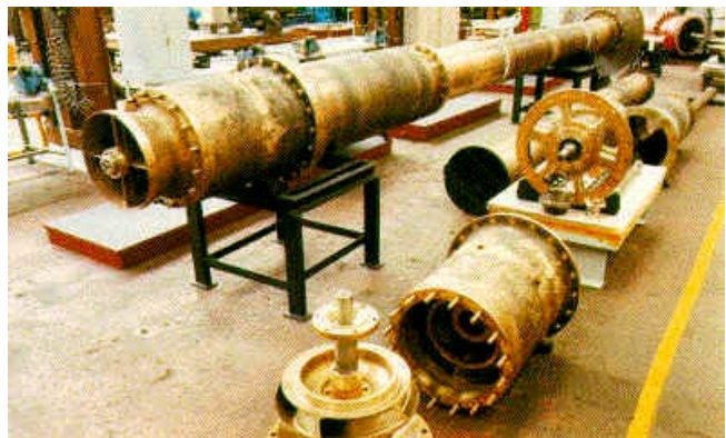
Figure 2 – Unit under construction – aluminium bronze components clearly visible
