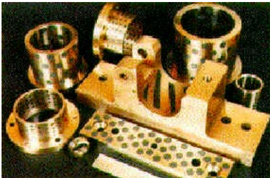
Figure 11 – Composite self-lubricating bearings with graphite inserts are available in a wide range of shapes and sizes for applications where conventional lubrication is difficult
