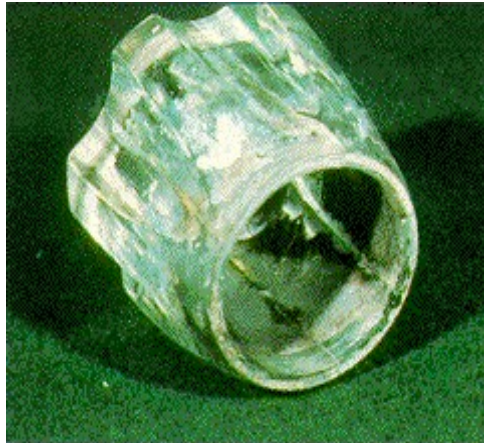
Substitutes for plastics - tap tops - material that appears to be a good substitute for brass has its own drawbacks
